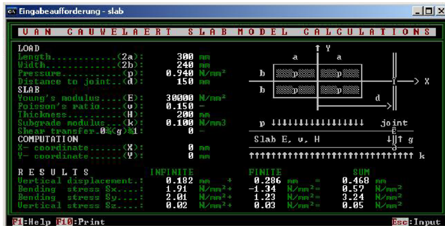
Fig. 8: Stresses and deformation when a load is applied to a 20 cm thick concrete slab on expansion resin with a ballast modulus of k = 0.1 and a wheel load of (5.5 \times 1.2 =) 6.6 tons
